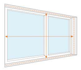
Should the windows or doors be sited where there is no reveal (particularly common on sliding sash windows) please measure between any surrounding architrave or trim and vertically to the bottom of any internal window board
