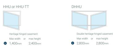
All windows are supplied fully assembled and ready to install. Units comprise of an aluminium outer frame joined to a seasoned hardwood timber surround.
